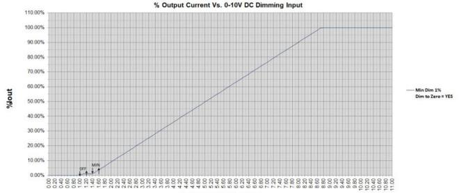
Dimming Input VDim(Vdc)
