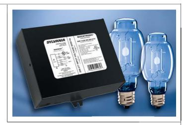
mechanical vibrations within the lamp structure resulting in an audible noise or acoustic resonance. Acoustic resonance issues may cause visual flickering, lamp cycling, shortened lamp life, and in extreme cases may result in non-passive failure. This low frequency square wave approach is robust with respect to acoustic stabilities and is immune to variations in lamp geometry, fill chemistry and mercury dose.
