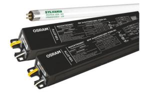
QUICKTRONIC PROStart T5HO 0.80BF ballasts operate PENTRON T5HO ECOLOGIC lamps. The ballast is tuned to provide a unique 0.80 ballast factor, providing 20% energy savings over conventional 2 lamp 54W T5HO systems.
