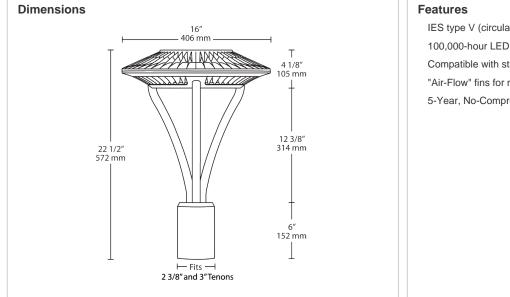
IES type V (circular) distribution 100,000-hour LED lifespan Compatible with standard 2 3/8" and 3" tenons "Air-Flow" fins for maximum heat dissipation 5-Year, No-Compromise Warranty
