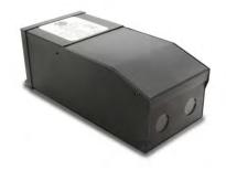
Magnitude's M300L12DC is the **most compact LED driver** on the market with a magnetic transformer core. It is equipped with 1 pushto-reset circuit breaker on the output, which protects both the load and driver. The driver is encased in a coated metal box that includes 2 knock-outs on the bottom to enable easy installation that **complies with electrical code** requirements.
