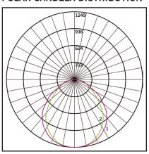
Maximum Candela = 1248.55 Located at Horizontal Angle = 0, Vertical Angle 0
