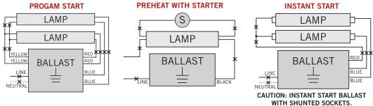
2. Re-wire fixture as shown below (maximum of 4 LED tubes per fixture).
