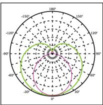
Maximum Candela = 1248.55 Located at Horizontal Angle = 0, Vertical Angle 0
