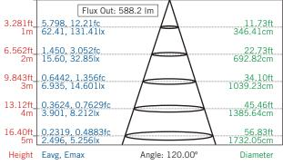
Note: The curves indicate the illuminated area and the average illumination when the luminaire is at a different distance
