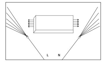
**4.** Access sign raceway/wiring box, and cut all ballast input and output wires as shown. Do not remove ballast if removal leaves opening in raceway.
