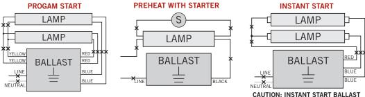
2. Re-wire fixture as shown below (maximum of 4 LED tubes per fixture).
