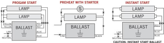
2. Re-wire fixture as shown below (maximum of 4 LED tubes per fixture).
