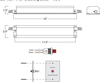
A Test/Monitor Plate with an illuminated test switch/charging indicator light is provided.
