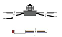
A test switch and charging indicator light is provided.
