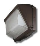
The WP 120 Watt is a rugged, durable LED wall pack, which is perfect for outdoor perimeter and area lighting. With a die cast aluminum housing and a vandal resistant, borosilicate glass lens, the WP 120 Watt will stand up to many years of punishing environmental conditions. High-efficacy, long-life LEDs provide both energy and maintenance cost savings compared to traditional, HID wall packs.
