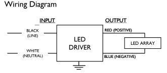
Input and output use lead-wires. Lead-wires are 18AWG 105C/600V solid copper
