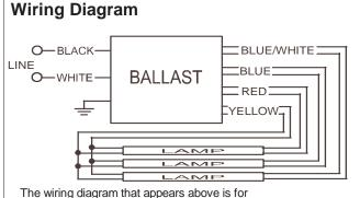
The wiring diagram that appears above is to the lamp type denoted by the asterisk (\*)
