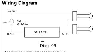
The wiring diagram that appears above is for the lamp type denoted by the asterisk (\*)
