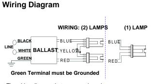
The wiring diagram that appears above is for the lamp type denoted by the asterisk  $(\sp{*})$
